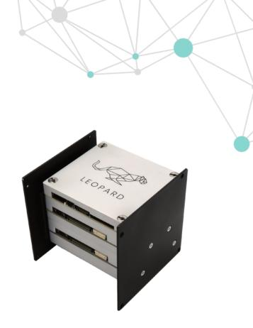
Leopard is integrated with a powerful FPGA to accelerate execution of deep learning algorithms and has a through put of up to **3 Tera Operations Per Second**. A number of hardware and software measures protect the computer against the influence of radiation.
